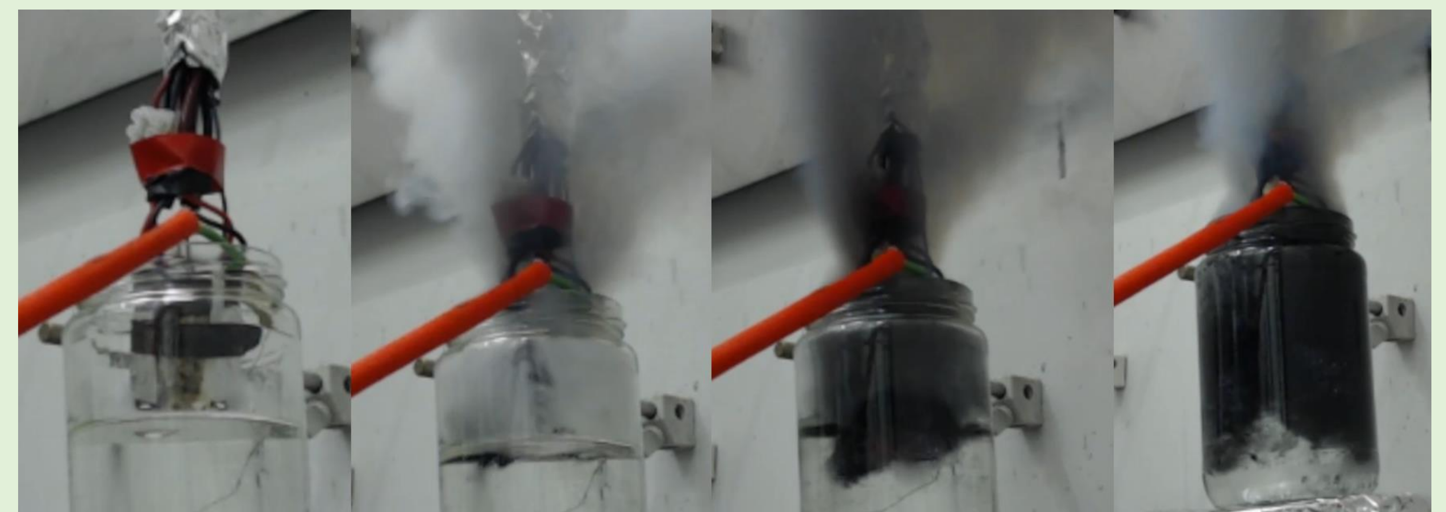
Figure 4: Emergency cooling of lithium-ion pouch cell. Immersion in coolant after first visible flame.
