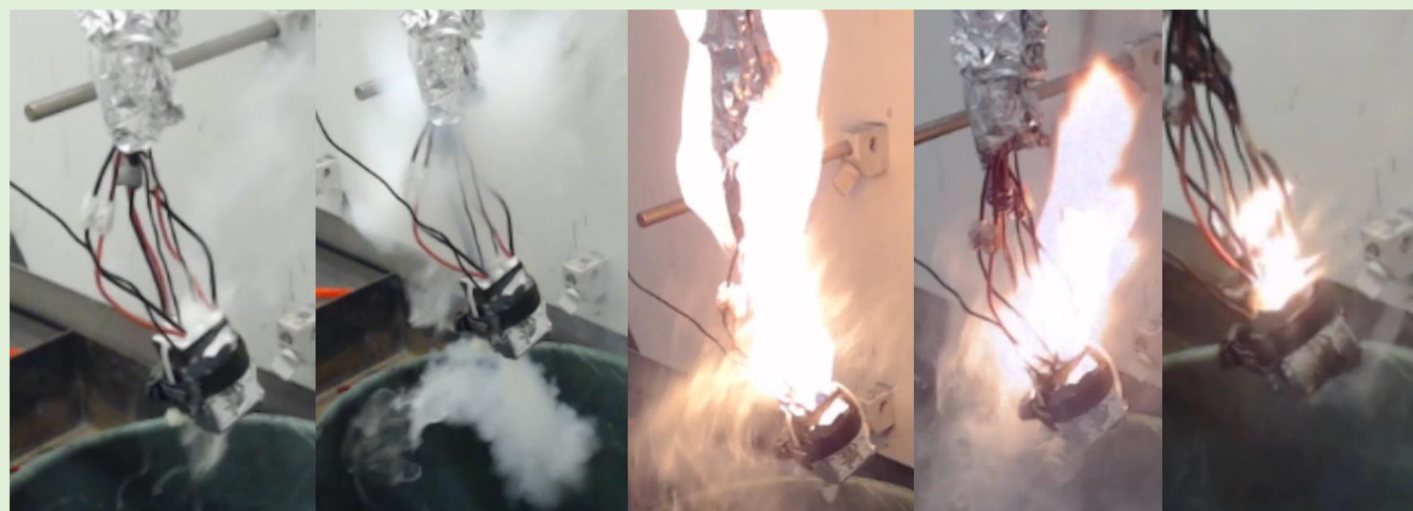
Figure 2: Thermal runaway of lithium-ion pouch cell.
