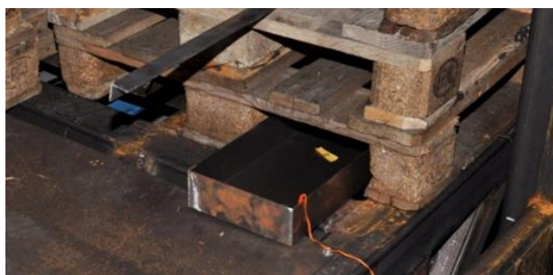
Figure 14. Pool for Class A - Euro pallet fire load with remote igniter (before sliding under the pack of pallets)
